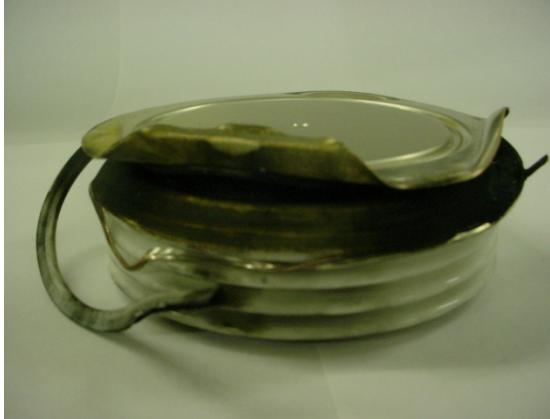
Fig. 8. Thyristor with arc shield finally failing at the cold weld due to internal pressure.
